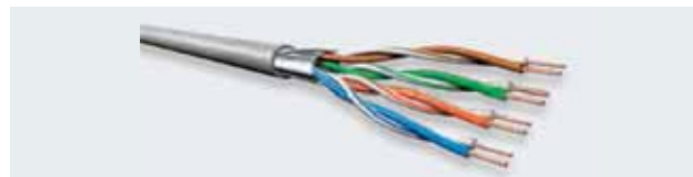
F/UTP: foil screened unshielded twisted pair; overall screen made of metal foil; also referred to as FTP cable
