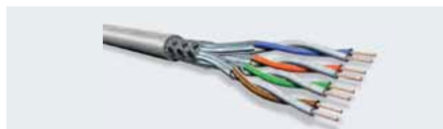
S/FTP: braid screened shielded twisted pair; overall braid screen made, pairs individually shielded by metal foil. Most common type of shielded cable; also referred to as PiMF (pairs in metal foil).
